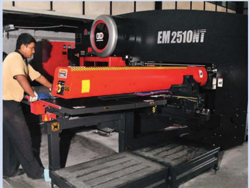
CNC AMADA '2510NT' Double Servo Turret Punch
