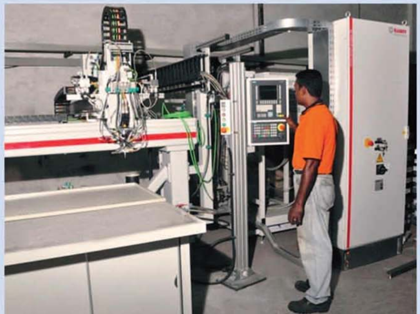
RAMPF Robotic Arm Gasketing Machine
